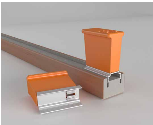
M-BLOCK-CD Tool to pre-mount U-FIX-CD or U-FIX-CDC to the backside of the ribs. Use a hammer.
